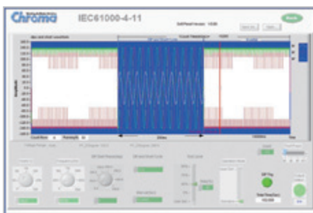
Voltage DIP, Short Interruption, Variation Test
